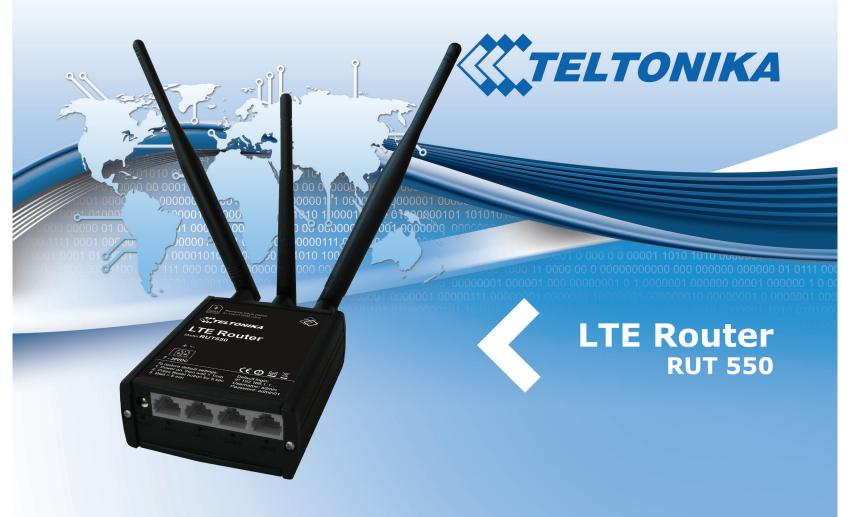
Teltonika RUT550 is compact LTE router with high speed wireless and Ethernet connections. Internal LTE modem can reach download rate of up to 100Mbps. Router supports the latest IEEE802.11n as well as IEEE802.11b/g standards and provides wireless receiving and transmitting rate of up to 150 Mbps. External antenna connectors make it possible to attach desired antennas and to easily find the best signal location.
